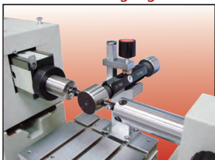
Plug gauge calibration with V-shaped carrier
