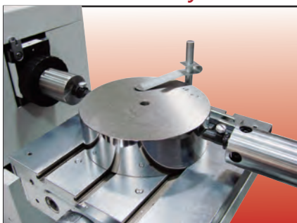
Cylinder gauge calibration
