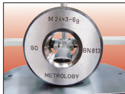
Inner thread gauge measurement
