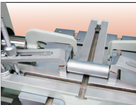
External snap gauge calibration
