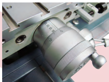
Vertical forward & backward micrometer head
